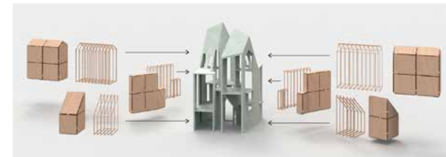
Wood Plug-in as Assembly Kit Into Concrete Skeleton
